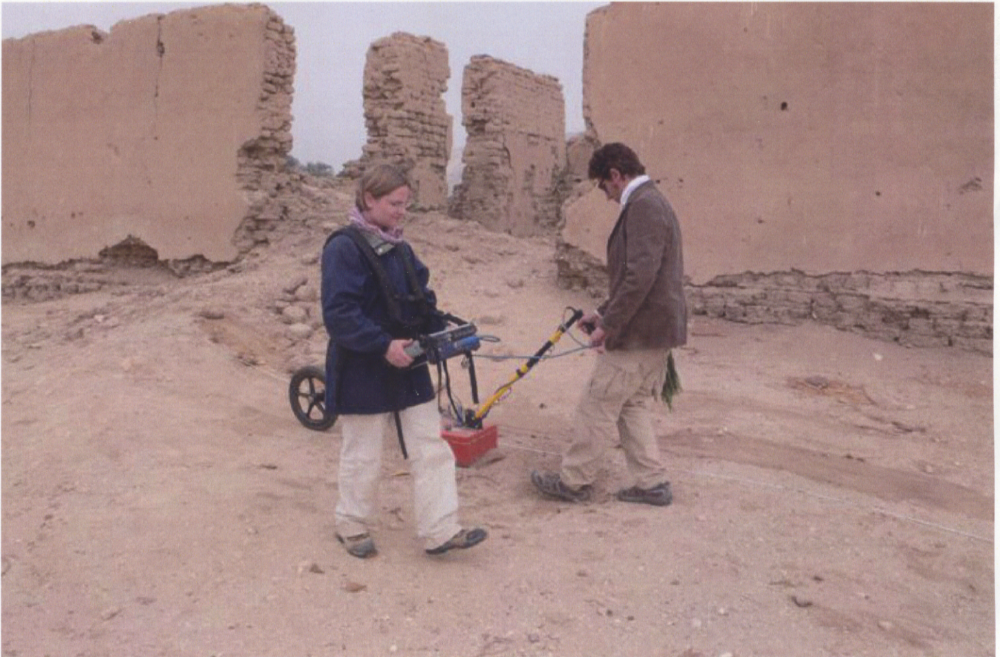
Fig. 9. The University of Arkansas geophysics team working with ground-penetrating radar equipment beside the old Pendlebury dig house at Amarna.
