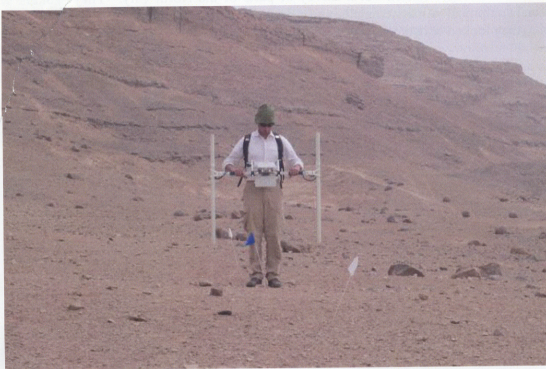
Fig. 10. Christopher Goodmaster calibrates the magnetometer at the North City
